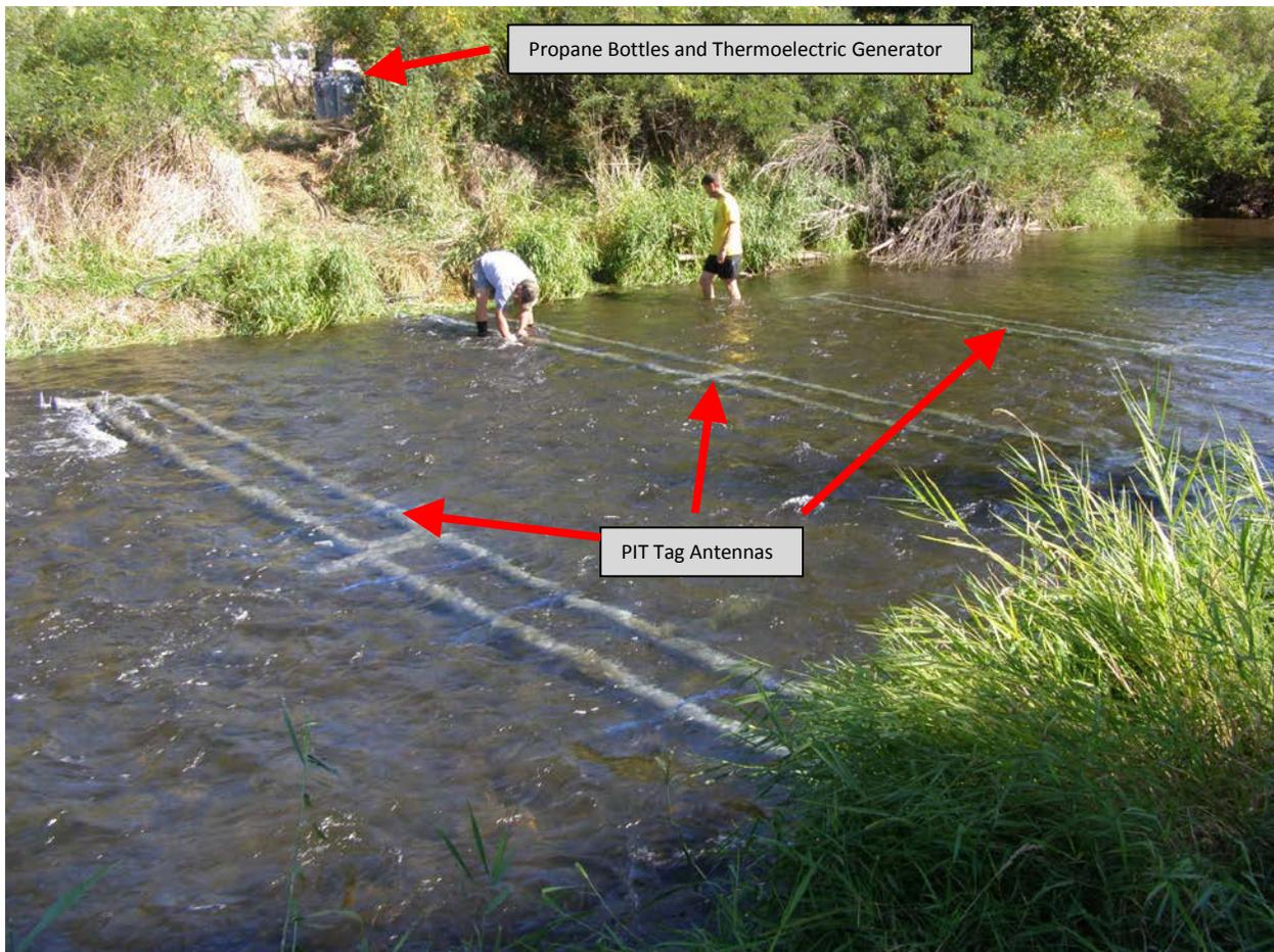
**Photo 1. Lower Tucannon River PIT Tag Array as redeployed in 2010. Three 15ft antennas that quit working were replaced during the summer of 2011 with 20ft antennas. The array now spans from shoreline to shoreline with three rows.**
